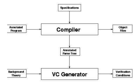
Figure 5.2: Prototype VC Generator Architecture
